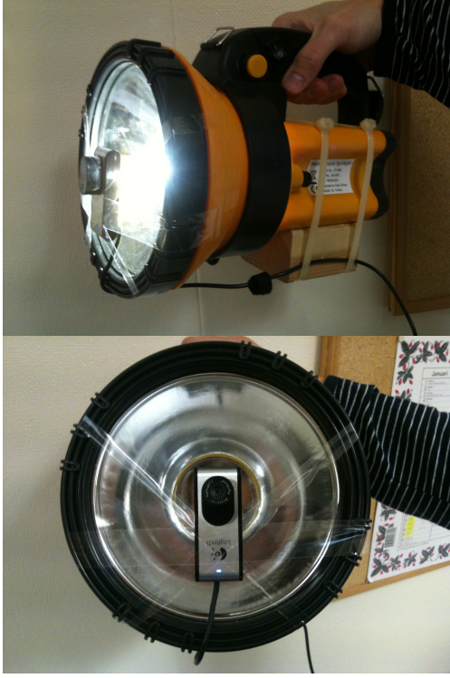
Fig. 1. Experimental setup: rechargeable spotlight and a webcam glued to the center of its frontglass.
