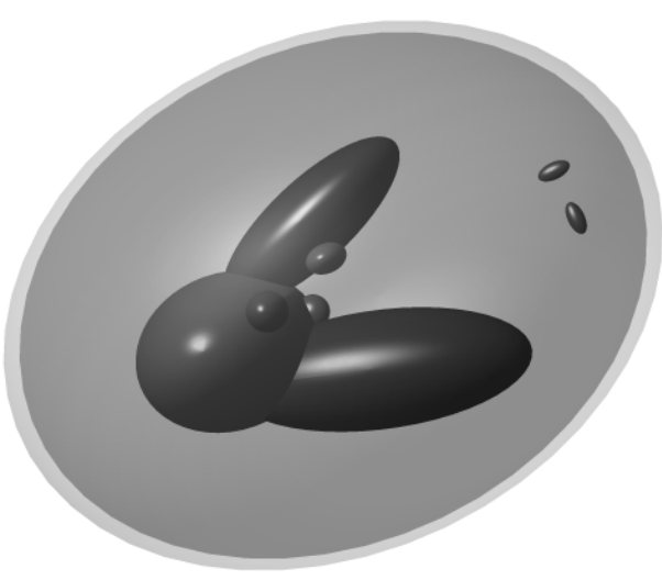
Fig. 4. A three-dimensional version of the Shepp-Logan phantom.
