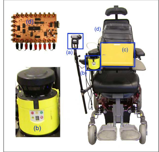
Fig. 1. Our electric wheelchair fitted with a) a camera (logitech 9000, 30fps), b) a SICK Laser scanner S300, c) a laptop (CPU Pentium M 1.6 GHz, RAM: 1GB) and built in sound unit, d) vibrotactile motors (8 coin-motors controlled by PWM generated by micro-controller).
